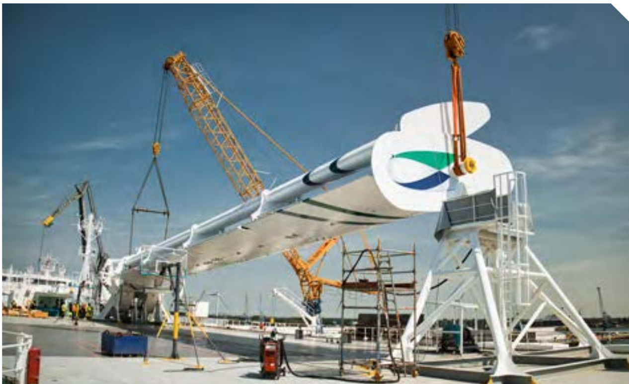
An Econowind's VentoFoil being readied for installation
