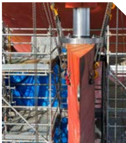
Removal of the damaged rudder (right) and installation of the repaired rudder (left)
