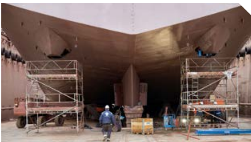
Above: Fugro Synergy was docked for a complete overhaul of its thrusters and propeller
