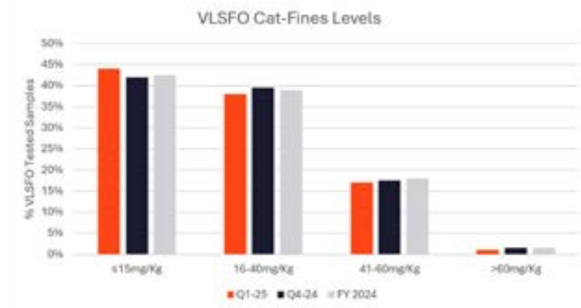
Figure 3: VPS tested VLSFO Cat-fine Levels
