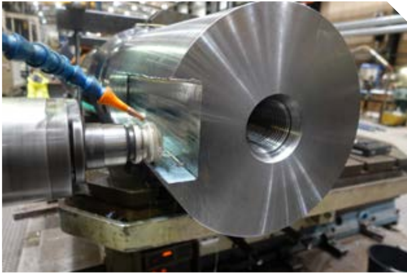
Manufacturing the new rudder stock
